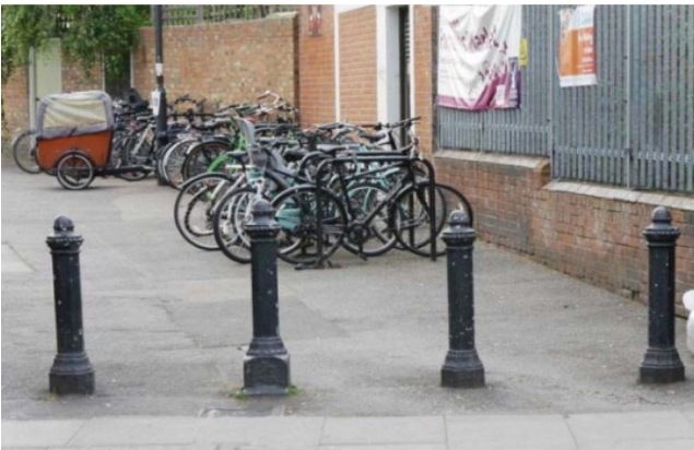
Bollards set closely together, making access difficult or impossible for non-standard cycles
